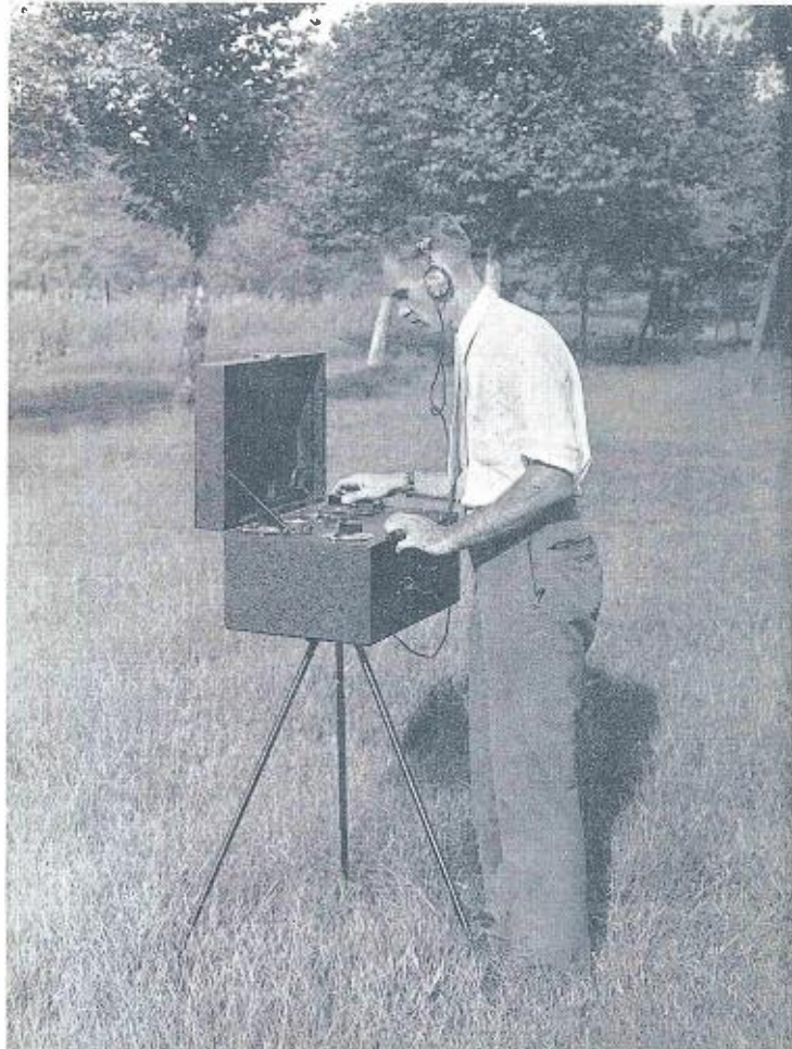
FIG. 4. NEW TYPE TMJ-21 FIELD INTENSITY METER BEING USED IN THE FIELD BY MR. GHIRING, RCA VICTOR ENGINEER. NOTE COMPACTNESS AND CONVENIENT TRIPOD MOUNTING.
